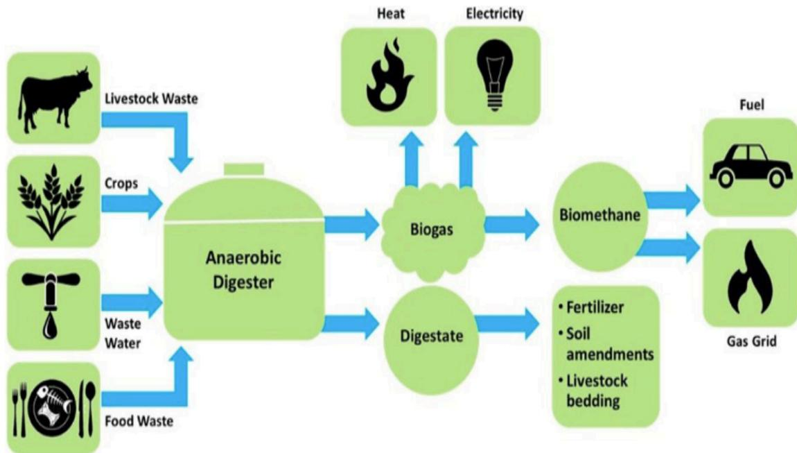
Figure 1: Anaerobic digestion process
